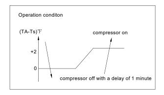
When TA $\leq$ TS (lasting 1 minute), compressor off When T1>TS+2°F, compressor on
