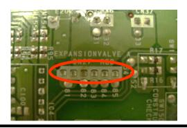
To ohm out the expansion valve, set your multi-meter to 'ohms' and conduct the tests using the chart.
