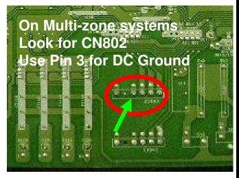
2. Test on all six solder points on the board and verify voltage reads 12-13 volts DC.
