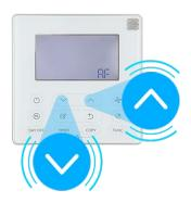
• Then press "V" or "A" to select "AF", press "Confirm" into test mode ,the "ON" stars to flicker.
