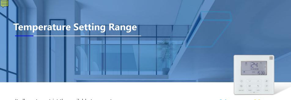
It allows to restrict the available temperature setting range of wired controller, for example, 24°to 28°. The room always remains comfortable with lowest energy consumption, which is useful in hotel, office, hospital and school. But you can still adjust cooling or heating temperature by remote control from 17°to 30°as always.
