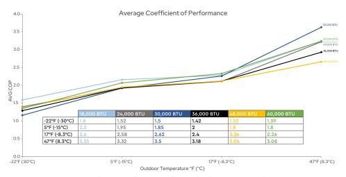
NRCAN and the Government of Canada define the Coefficient of Performance (COP) of a heat pump as the ratio between the rate at which the heat pump transfers thermal energy (in kW), and the amount of electrical power required to do the pumping (in kW). For example, if a heat pump used 1kW of electrical energy to transfer 3 kW of heat, the COP would be 3.
